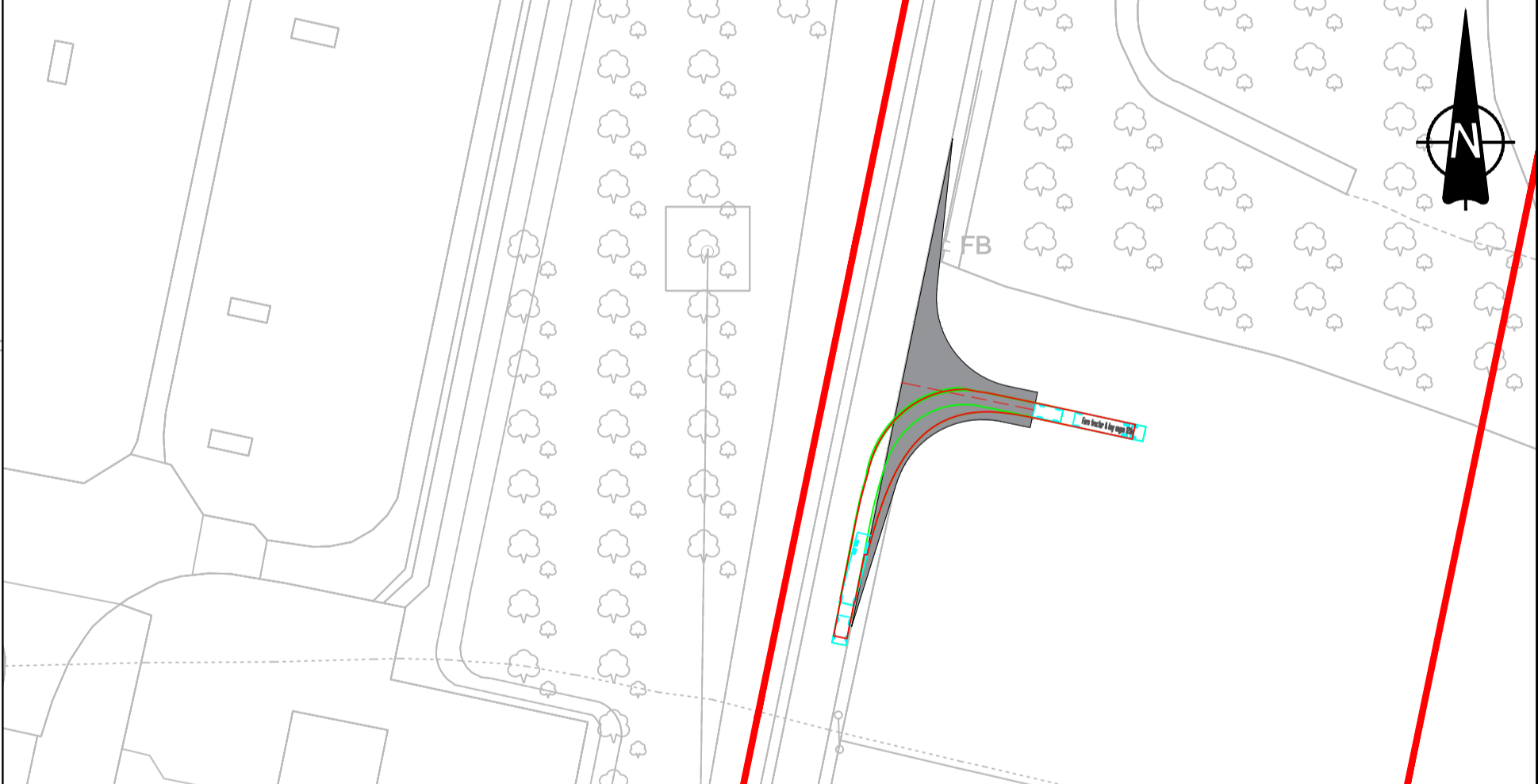
INSET C: ARTICULATED VEHICLE MANOEUVRE HEADING OUT OF ACCESS, LEFT TURN ONTO NEW ROAD LANE HEADING SOUTH - SCALE 1:1000
